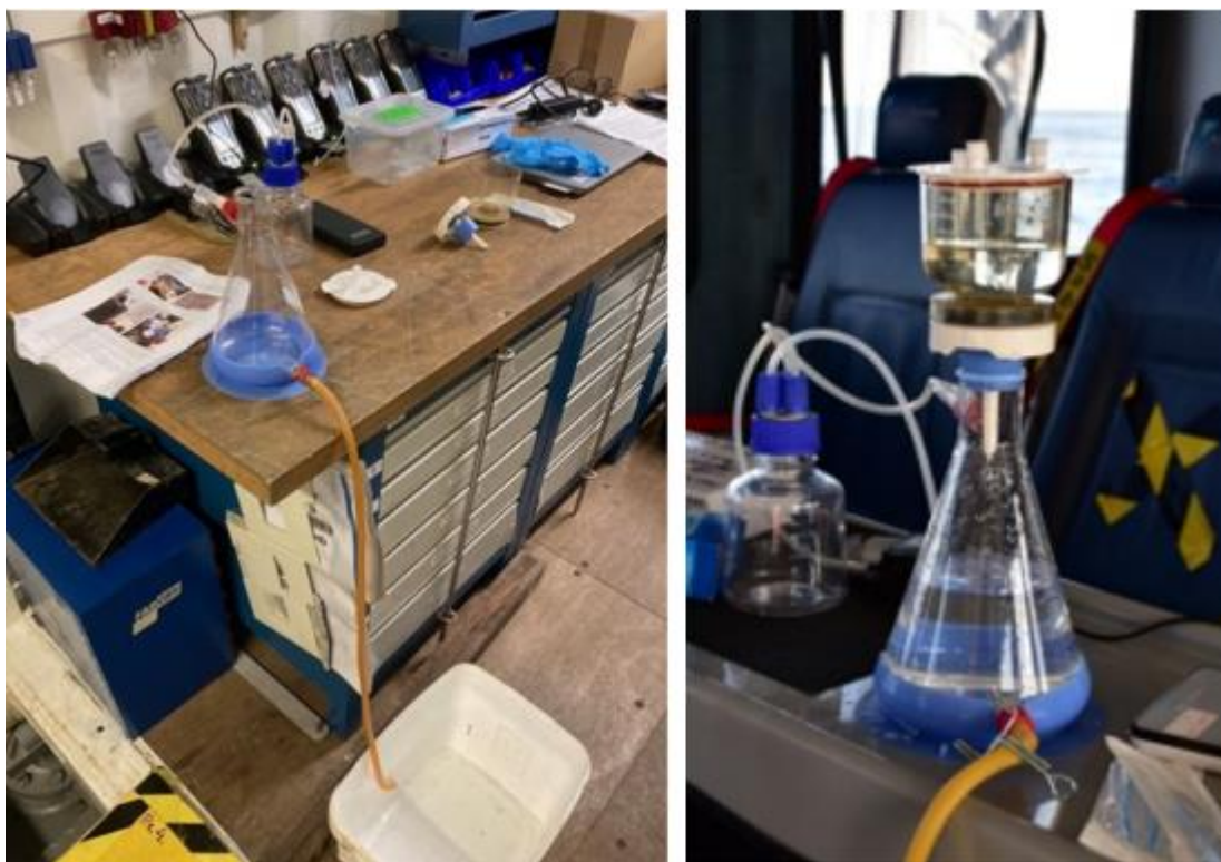
Figure 16. Water filtration kit used to filter eDNA from seawater samples.
