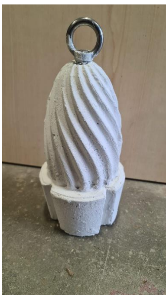
Figure 5. The small concrete reef plug elements which sit atop the ExoLodges, including close-up of patterned design.
