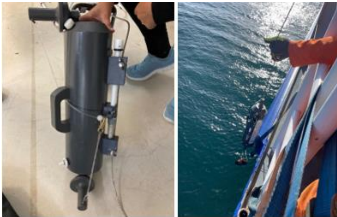
Figure 15. Niskin bottle used for water sample collection for eDNA.
