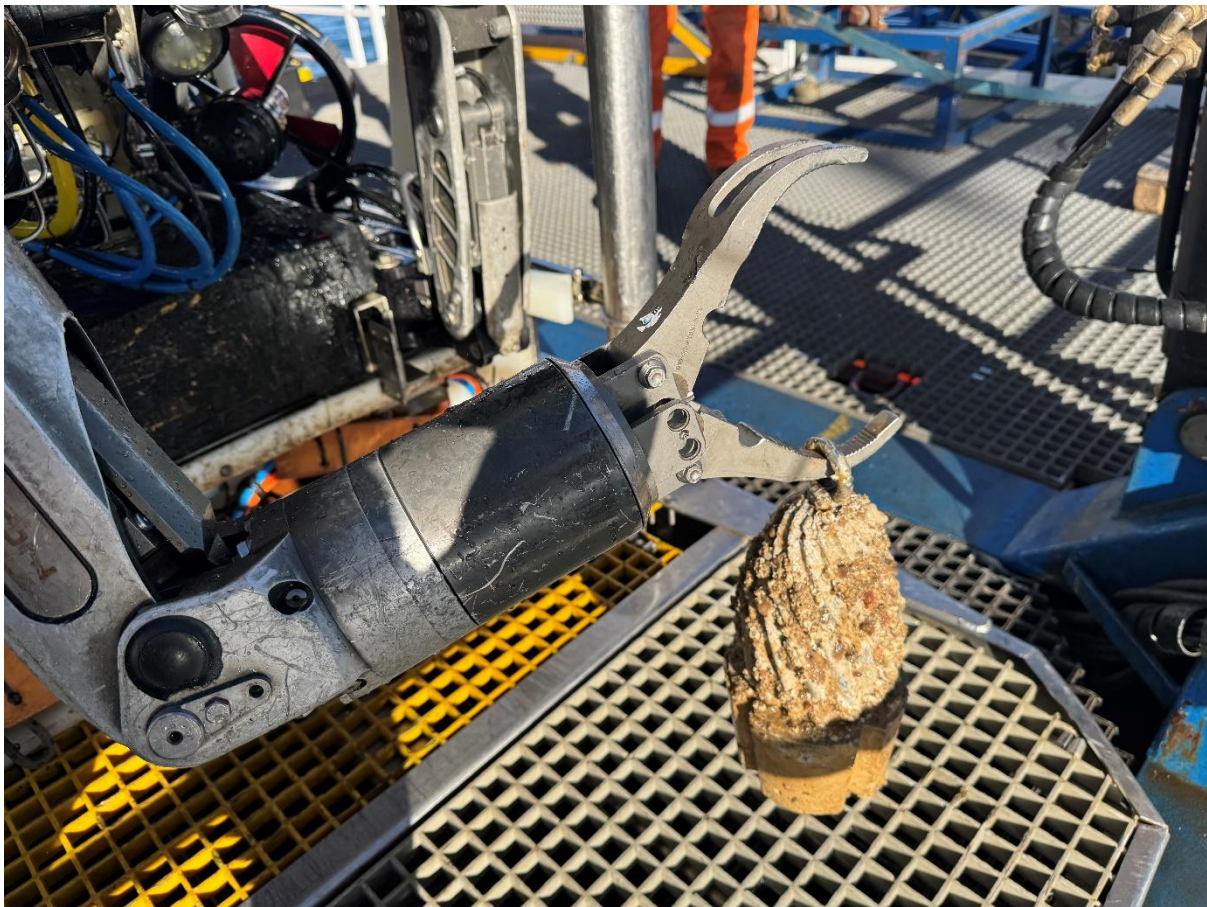
Figure 13. The reef plug recovery using a work-class ROV during T1 monitoring in September 2025.
