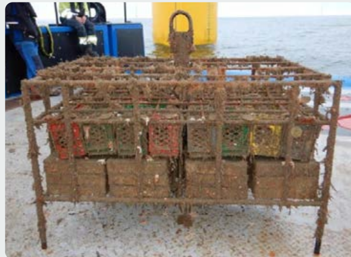
One of the experimental cages after nine months on the seabed
