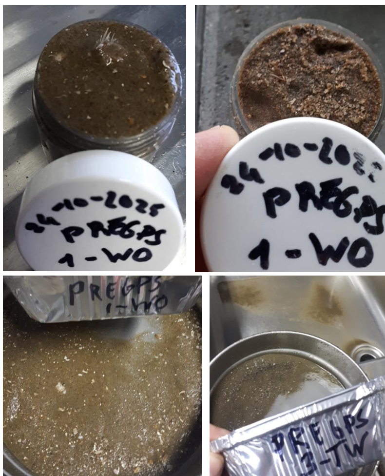
Figure 22 Photographs of subsamples. Upper left: photo of subsample 1-WO. Note the presence of surface-sticking small spikes belonging to a benthos species. Diameter of the pot is about 4 cm, for scale. Upper right: photo after air drying a month later, from which the coarse sand grains and shell fragments can clearly be seen. Lower left: wet sieving of the very sandy 1-WO sample to separate sand/mud. Lower right: idem, for the muddy 3-TW subsample; note the fines in the drain.
