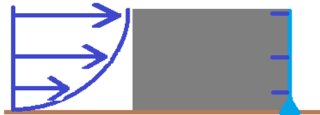
Figure 10: Overturning moment, discretized method
