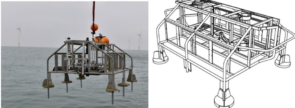
Figure 5: MIXLander frame. Left: during deployment. Right: technical drawing (first version).
