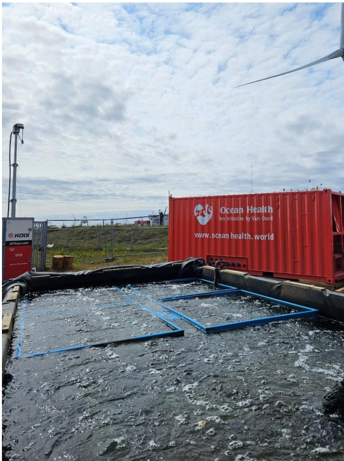
Figure 2-4. View of the remote setting facility. In the foreground the remote setting container with four tipping buckets. A small part of the rock bag is visible in the right-hand corner, the remainder of the rock bag is obscured from vision by the air bubbles. The water treatment container is visible on the right-hand side.
