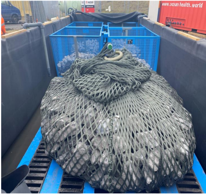
Figure 2-3. View of the remote setting container before adding water. The rock bag is visible in the foreground, and the tipping containers in the background, all filled with rocks.
