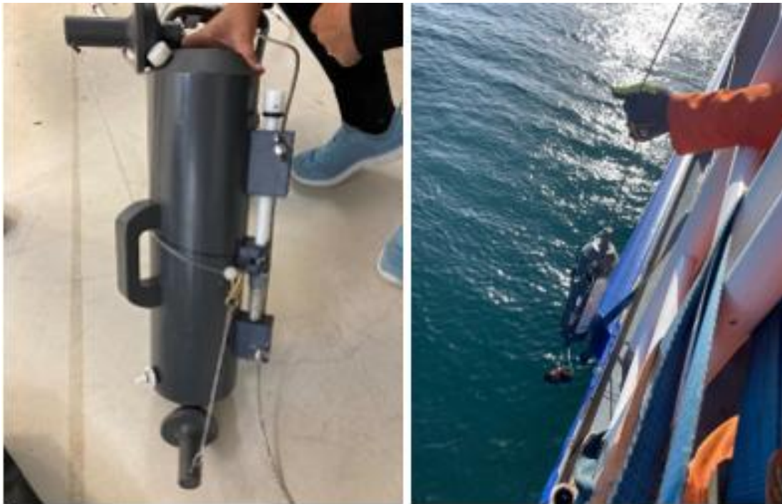
Figure 10. Niskin bottle used for water sample collection for eDNA
