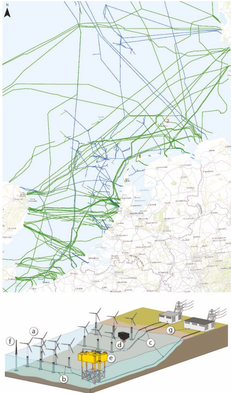
Figure A.6 Top: cables (green) and pipelines (blue) in the DCS (from Snoek et al 2016). Bottom: Typical layout of a OWF, a) wind turbines b) infield cables c) export cables d) transformer station e) converter station f) meteorological mast g) onshore station (figure from Rodrigues, 2016).
