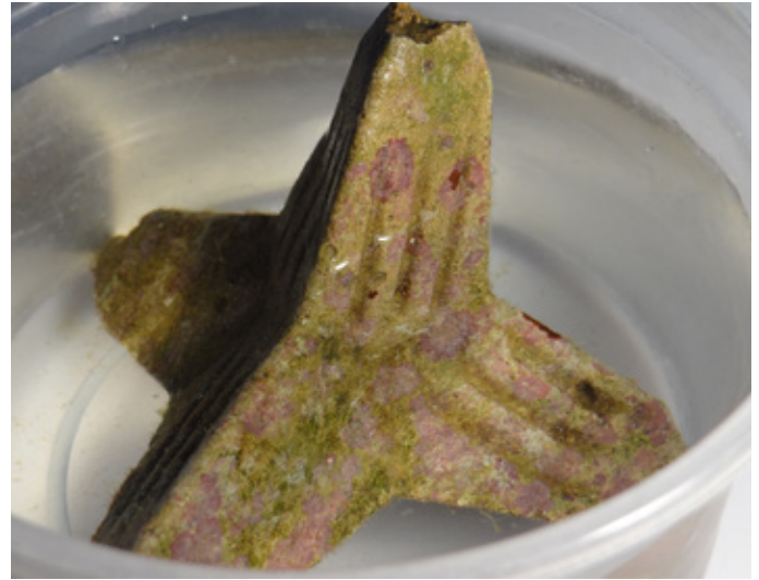
Figure 26: Biofilm on a concrete unit (photo: SECORE).
