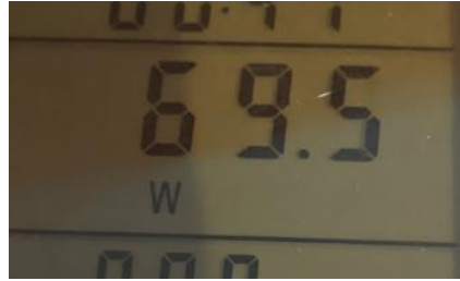
Figure 4: Power consumption 220V pump
