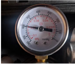
Figure 3: pump inlet closed gives approx. -0.06 MPa or -600mmHG
