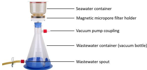
Figure 1: MF31 filtration apparatus with part description
