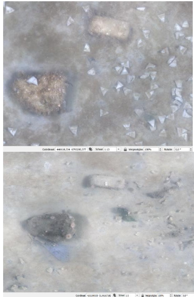
FIGURE 39. TOP: REFERENCE POINT T0 (PROPER VISION). BOTTOM: REFERENCE POINT T2 (POOR VISION). THE GRID OF T0 AND T2 OVERLAPS AT THE EXACT GPS COORDINATES, USING MULTIPLE NON-MOVEABLE REFERENCE POINTS LIKE ROCKS VISIBLE IN THESE SCREENSHOTS.
