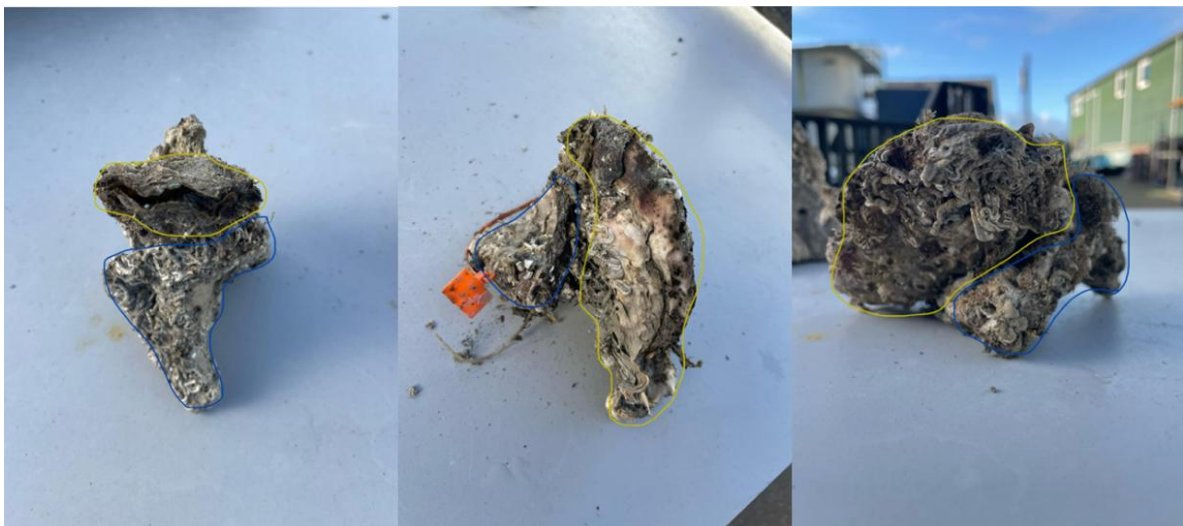
FIGURE 44. PICTURES OF THE REEFBOOSTER RETRIEVED FROM THE PORT WITH OYSTERS ATTACHED. THE OYSTERS ARE SURROUNDED IN YELLOW AND THE REEFBOOSTER IS SURROUNDED IN BLUE (THIN LINES).
