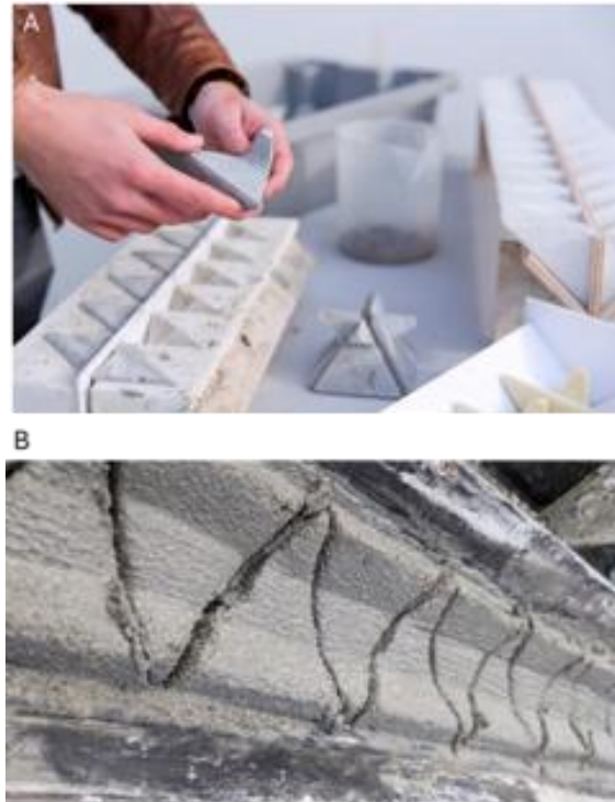
FIGURE 18. PICTURES OF THE PRODUCTION PROCESS OF THE DIFFERENT REEFBOOSTER DESIGNS. A SHOWS DESIGN A, AND B SHOWS DESIGN B.
