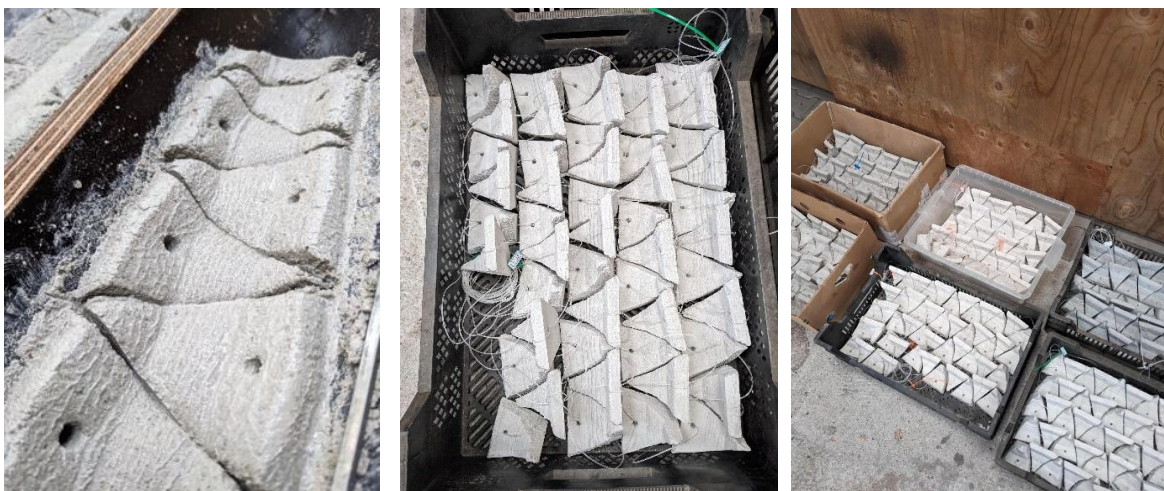
FIGURE 41. DESIGN B OF THE REEFBOOSTER, PRODUCED BY ATS, WITH A HOLE FOR THE NYLON LINE TO PASS THROUGH.
