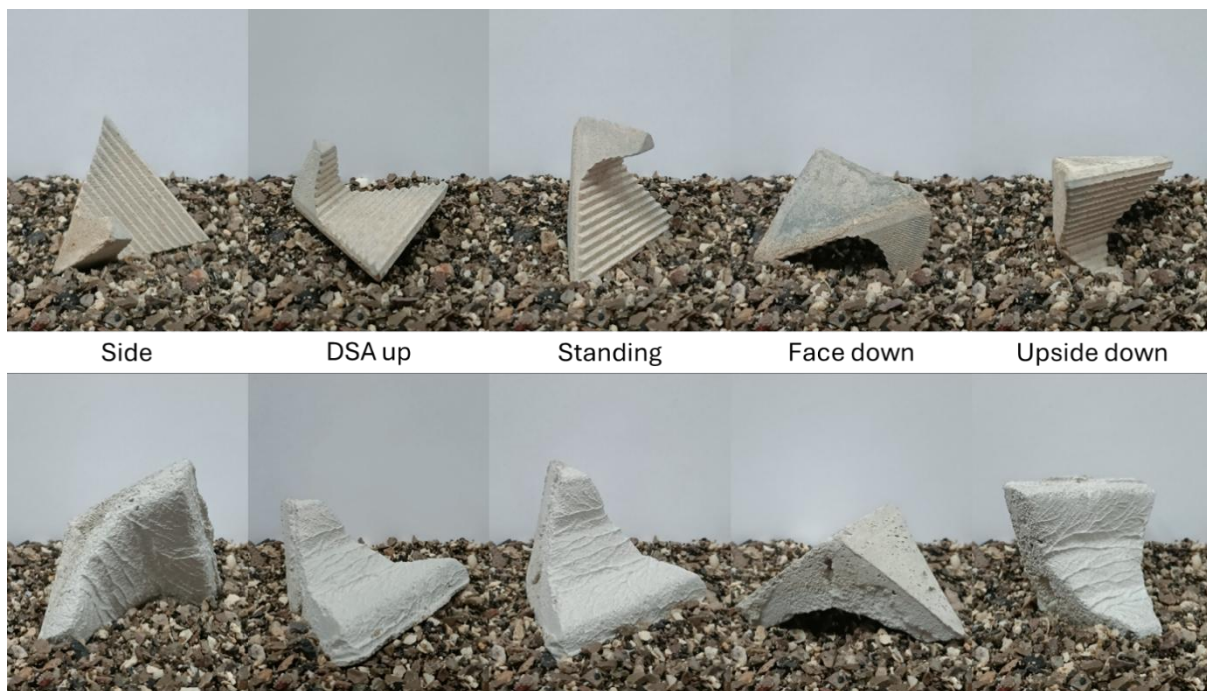
FIGURE 35. LANDING POSITIONS OF REEFBOOSTER DESIGN A (UPPER ROW PICTURES) AND REEFBOOSTER DESIGN B (LOWER ROW PICTURES) ON A COARSE SEDIMENT SURFACE WITH THE DEFINITIONS (SIDE, DSA UP, STANDING, FACE DOWN, UPSIDE DOWN).
