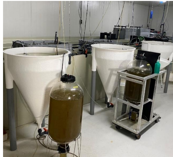
FIGURE 5. OVERVIEW OF LARVAL REARING SETUP IN THE HATCHERY OF BLUELINKED. THE WHITE CONICAL TANKS ARE THE NURSERY TANKS.
