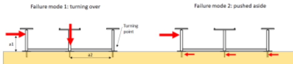
Figure 5: Failure mechanisms considered (from WaterProof, 2020).
