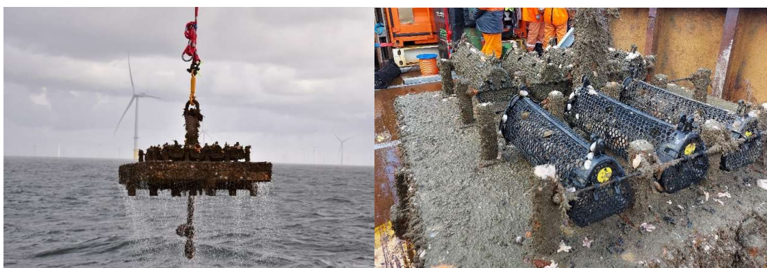
Figure 6. Hoisting of the oyster table (left) and oyster table on deck, with both (yet unsampled) baskets covered in marine growth and cleaned and newly attached baskets (right).
