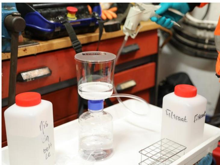
Figure 2-10: eDNA filtration set-up on the research vessel.
