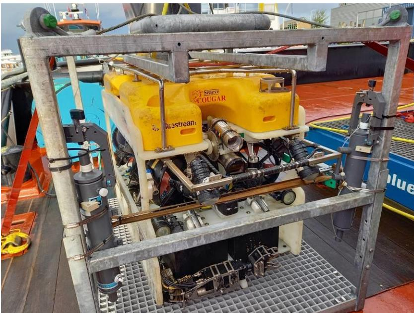
Figure 2-9: ROV in cage, with 2 Niskin bottles attached vertically.
