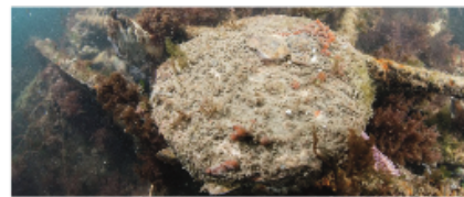
Disc of BESE-reef paste in the Dutch North Sea. After one month flat oyster spat ( Ostrea edulis ) colonized the structure
