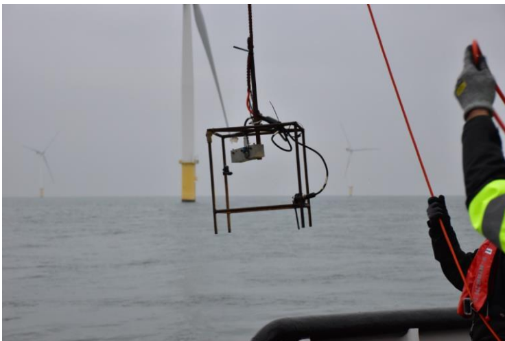
Figure 3.4 Drop cam monitoring prior to deployment
