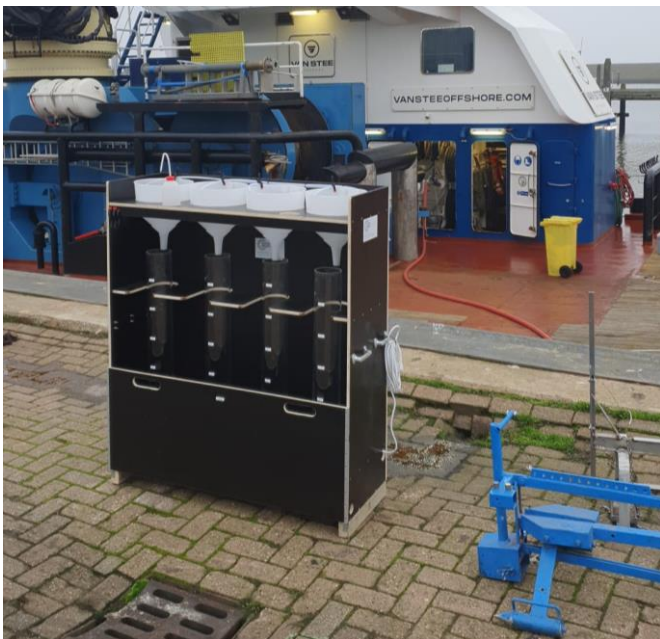
Figure 2.9 Water sampling cabinet and Blue Marlin measurement fish of WaterProof
