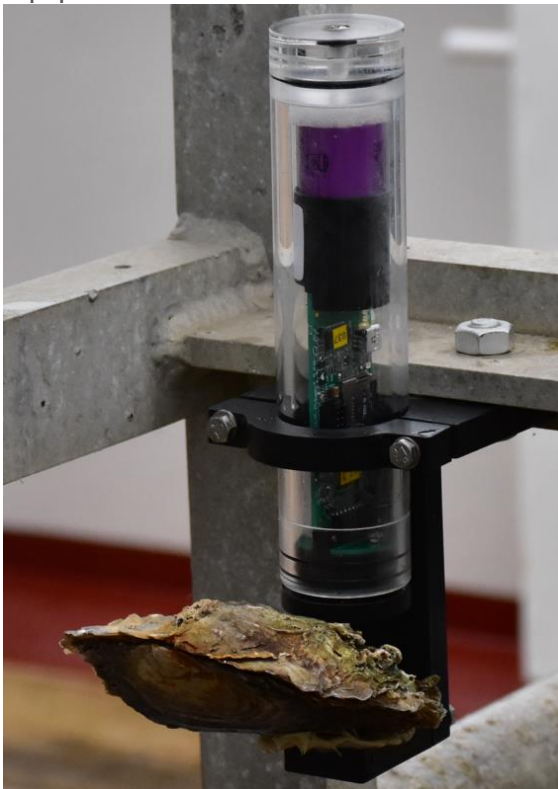
Figure 1: Valve position sensor with mounted oyster on measurement frame
