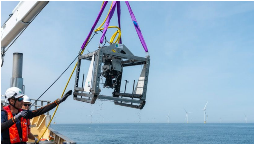
Photo 2: the dropcam system just before deployment
