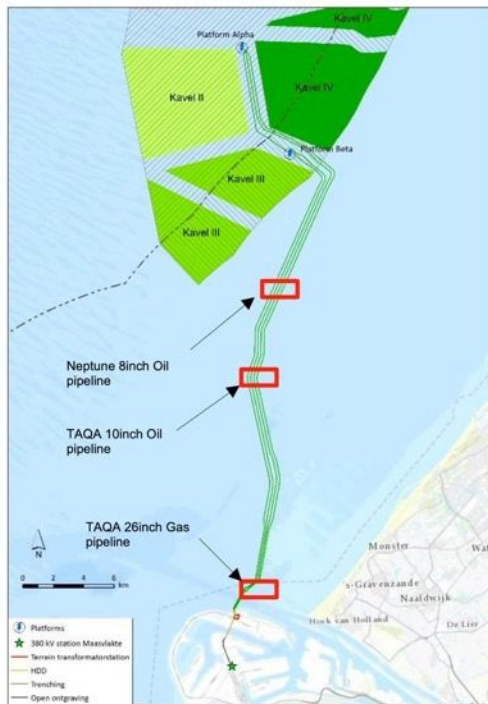
Figure 1: Locations of the cable crossings
