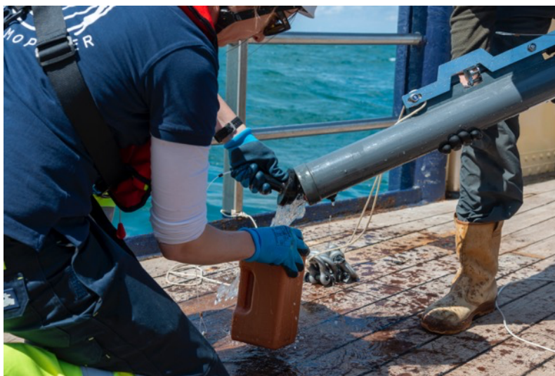
Photo 3: eDNA sampling with a Niskin bottle water sampling device.
