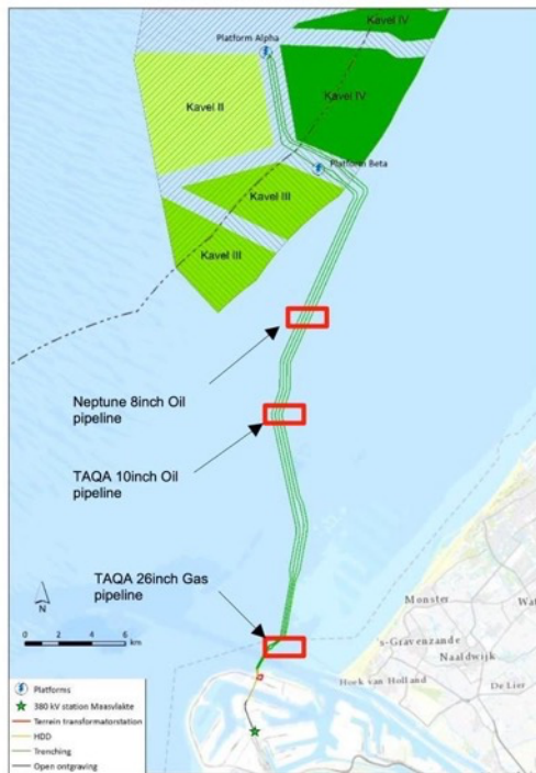
Figure 1: Locations of the cable crossings
