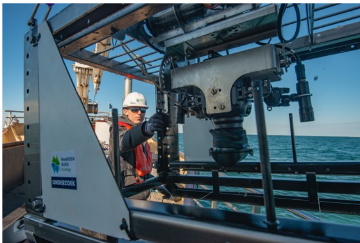
Photo 2: The 4K camera system which was used for image acquisition
